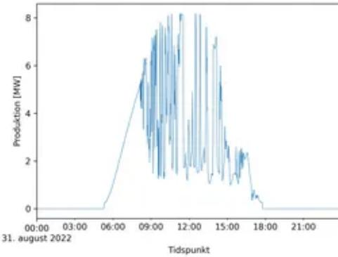
That's how jagged the production curve of a large Danish solar energy plant was on a slightly cloudy day in August this year.
